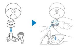
Remove the spool cap and place the spool of thread for the bobbin onto the spool pin.
