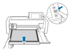
The mat is fed in to complete the preparations for cutting.
