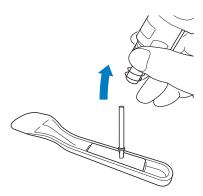
(For Rotary Auto Blade Holder) Hold the shaft section of the rotary auto blade, and remove it from the holder.
