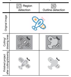
3 Select the detection method, and then touch the "OK" key.
