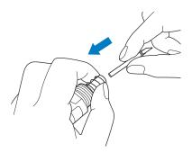
Twist on the holder cap to attach it to the holder.
