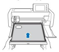
After selecting the cutting/drawing pattern, touch in the mat layout screen to start the background scanning function.
