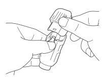
2 Remove the cap from the pen, and then insert the pen into the pen holder with the point down.
