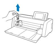
4 Use a commercially available brush to clean around the feed slot and the carriage.
